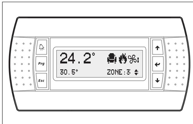
The display is an LCD 4 lines x 20 columns. The quantities and the information about the operation of the unit are alternated in the form of subsequent screens, named.
